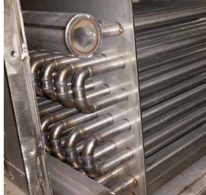
MS thermo oil heat exchanger for steam generation.
